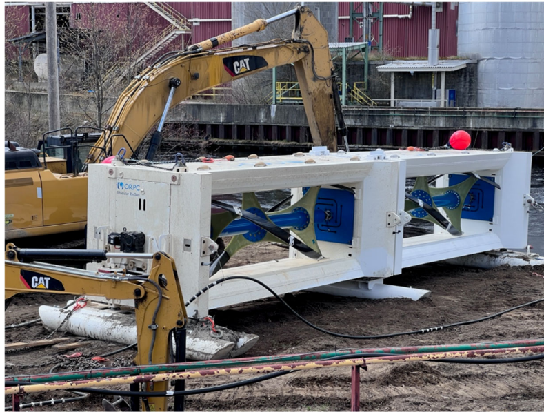
Figure 2: Modular RivGen power system (two horizontally connected devices), Millinocket, ME.
